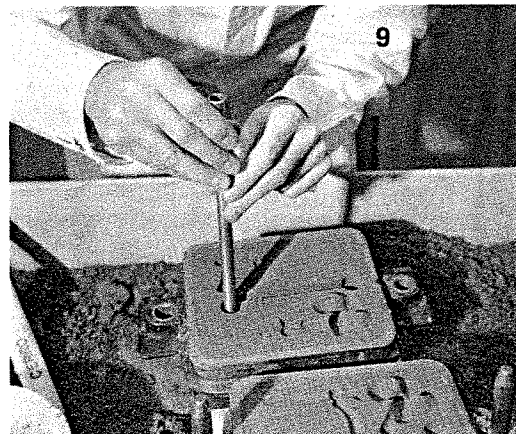
Making holes in cope for sprue and riser.
