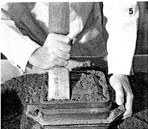
Peening sand against vertical sides of drag.
