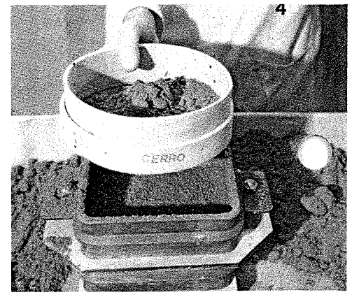
Riddling one-inch layer of sand over all pattern surfaces.
