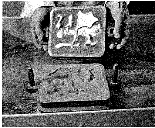
Cope removed from flask showing "gate" of castings.
